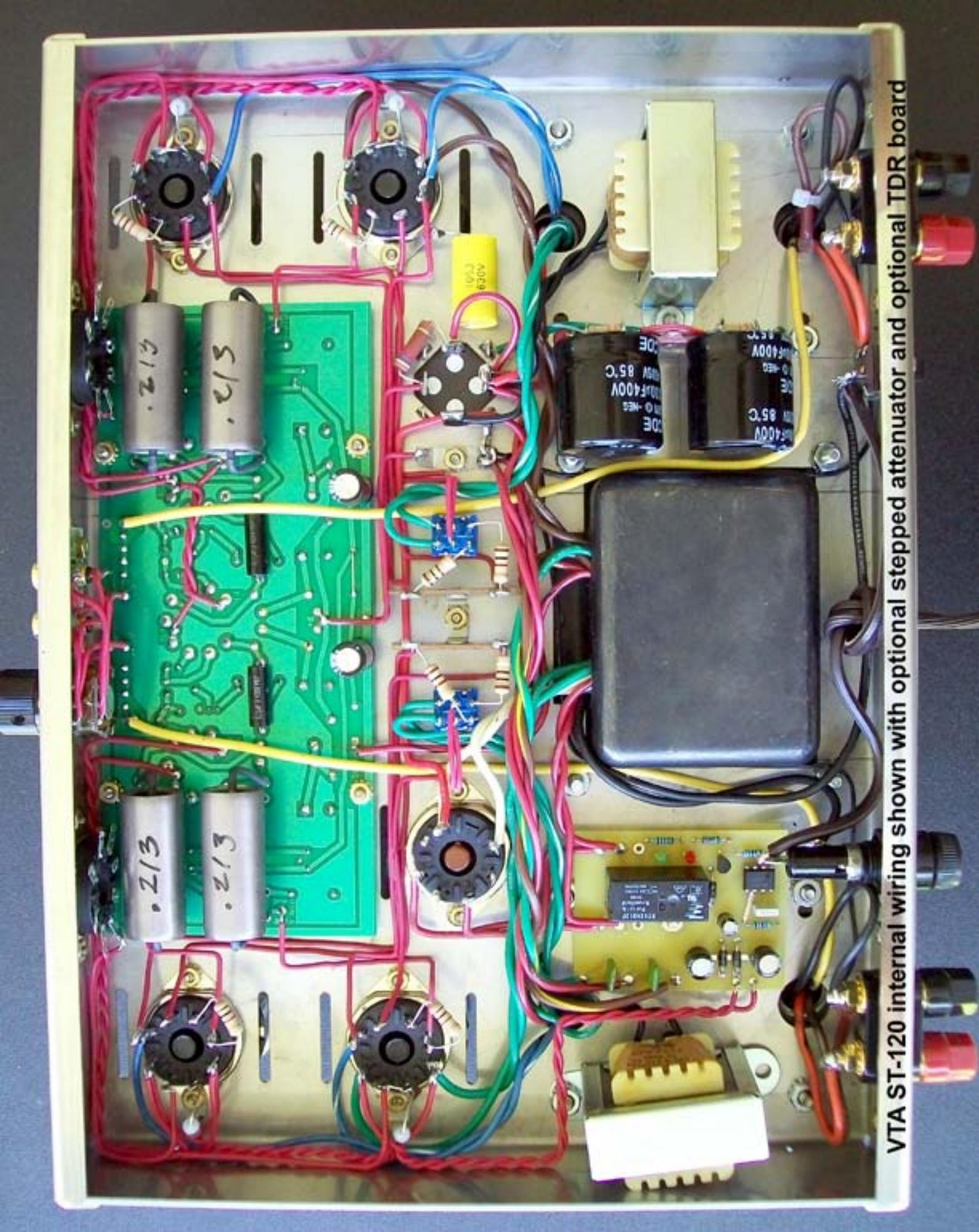
VTA ST-120 internal wiring shown with optional stepped attenuator and optional TDR board
